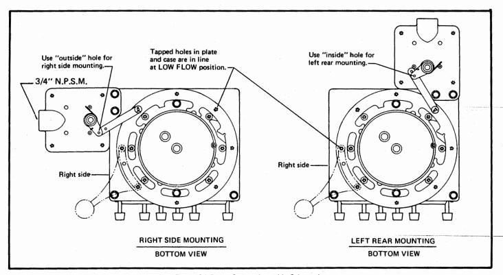
Figure 6-5 Preset Switch Assembly Schematic
